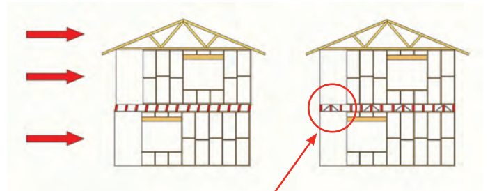
Additional vertical diagonal (shear) bracing
