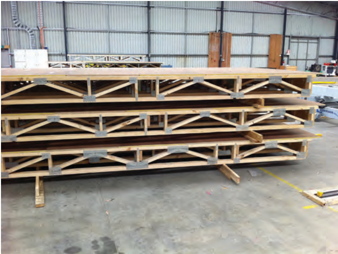
Stacking cassettes flat, level and dry
