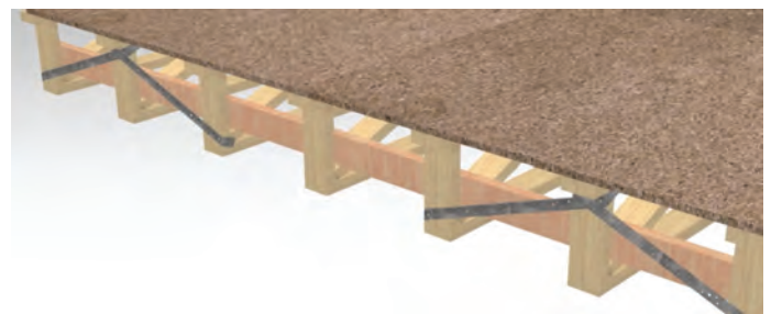
Lateral tie end bracing
